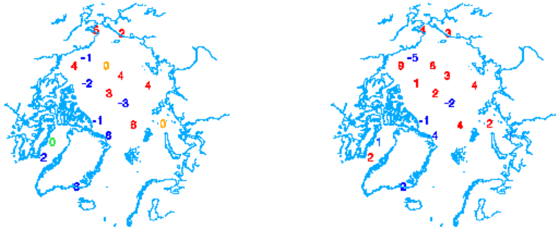
Figure 1. The two-metre temperature in the Arctic at 12 UTC on 5.12.2003: left panel – GME analysis using the new ice model, right panel – ECMWF analysis. Numbers show computed minus observed two-metre temperature difference (in K).
