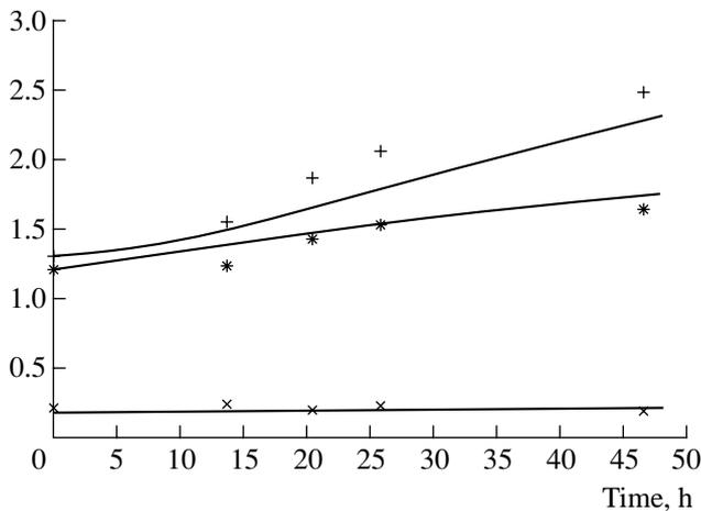
**Fig. 2.** Time variations in the CML lower boundary depth  $h$ , water temperature  $\theta_m$  in the CML, and the surface layer depth  $\delta$  for Lake Vendyurskoe during the period of penetrative convection. Curves correspond to the model data, and the symbols (pluses, asterisks, and crosses) correspond to the observational data on mixed layer depth, temperature, and surface layer depth, respectively.
