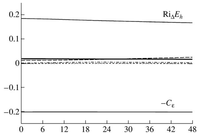
**Fig. 3.** Terms of the entrainment equation (12) as time functions. Solid lines at the bottom and at the top denote  $-C_\epsilon$  and  $Ri_\Delta E_h$ , respectively. The rest of the lines (from bottom to top): short-dash line corresponds to  $2/5 C_e D e$ , dotted line corresponds to  $-C_e E_\delta$ , dot-and-dash line corresponds to  $C_e E_h$ , dashed line corresponds to  $C_w Ri_N^{3/2} [\Delta h / (h - \delta)]^3$ , and heavy line corresponds to  $R$ .
