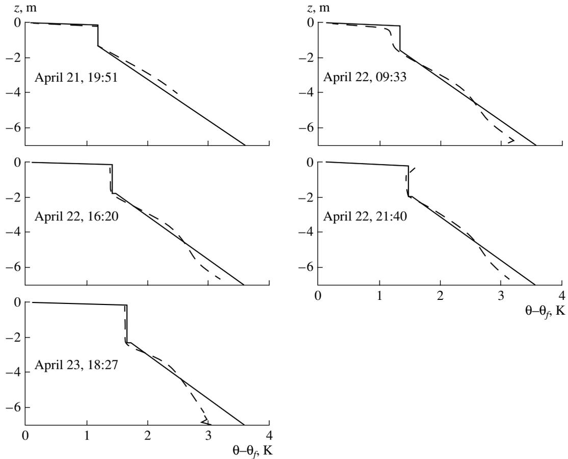
**Fig. 1.** Sequential temperature profiles for Lake Vendyurskoe within the period of penetrative convection. Solid lines correspond to the profiles calculated on the basis of the model proposed, and dashed lines correspond to the observational data. Dates and local time are indicated in the left parts of the figures. The observation point depth is 7.7 m.
